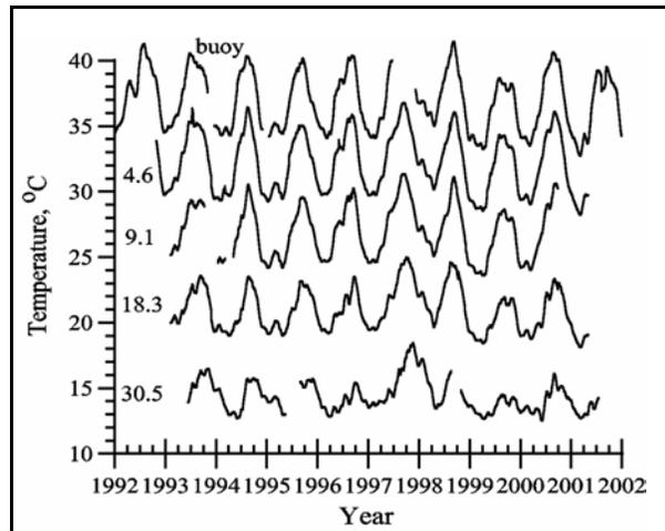
Figure 2. Averaged temperatures by depth measured by both the thermograph array off Santa Catalina Island and the Santa Monica Basin buoy, 1992-2001. All traces except the 30.5 m depth are offset from adjacent ones by 5° C.
