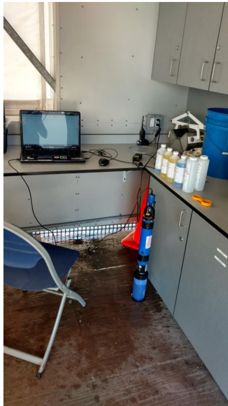
Figure 3-1. Laptop connected to sonde via cable interface
