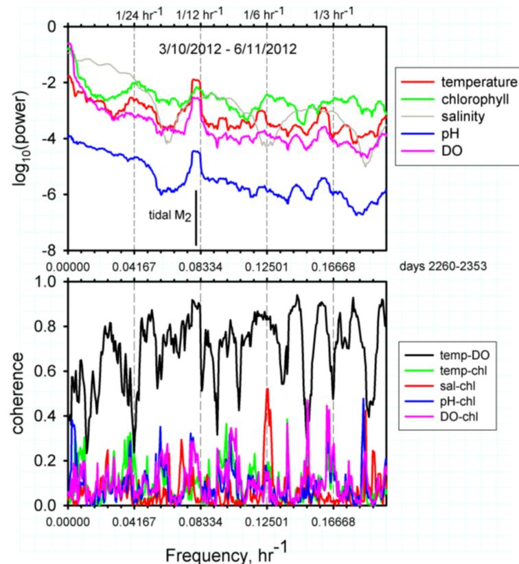
Power spectral densities of temperature, chlorophyll, salinity, pH and dissolved oxygen of CMS measurements made at the Wrigley Marine Science Center reserve from April – May 2012.
